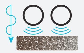
0.5 mm amplitude for sub-structure applications
