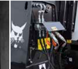
Auxiliary hydraulic line on boom head with FCS*
