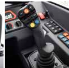
Smart joystick with Boom float and bucket shaking
