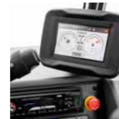
5" display with Bluetooth radio, microphone &amp; loudspeakers
