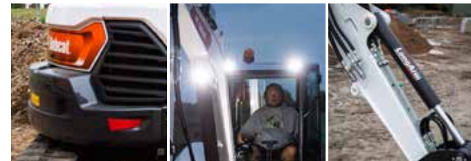
Heavy counterweight LED lights set Long dipperstick
