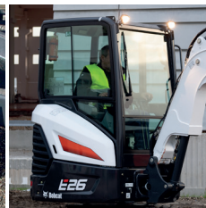
TOPS/ROPS/FOPS cab with heater
