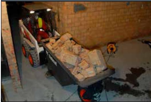
Dumping Hopper: Includes 8.5 x 12 Bobcat Heavy Duty Tire. Tire assembly to be installed on Dumping Hopper.
