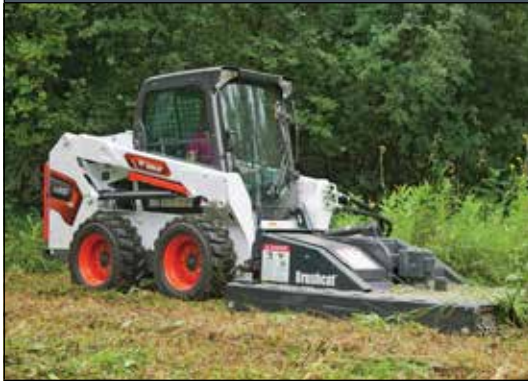
Brushcat™ Rotary Cutter: Comes standard with a 7 cm Offset Blade and Front Wheels. Cutting height of 7.6 cm.
