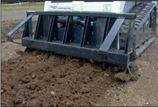
Scarifier: Includes 2 Depth Guides and 5 teeth.
